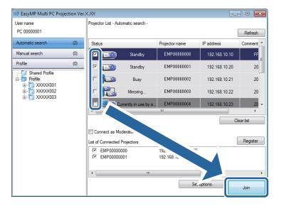
A projector mirroring group is formed and the same image is projected from multiple projectors.
